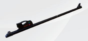
Electronic gauge is designed for measuring back-to-back distance of railway, metro and tram wheels in the course of checkup, examination, repair and formation of wheel sets.
